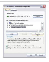
Select "Obtain an IP address automatically" and "Obtain DNS server address automatically". Click "OK" to save the configurations.
