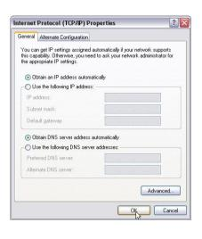
Or select "Use the following IP address" and enter the IP address, Subnet mask, Default gateway as shown right. Of course, you need to input the DNS server address provided by your ISP. Otherwise, you can use the Router's default gateway as the DNS proxy server. Click "OK" to save the configurations.
